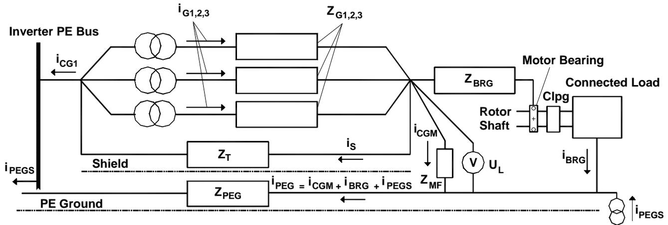
Fig. 9b Cable Equivalent Circuit<sup>12</sup>
