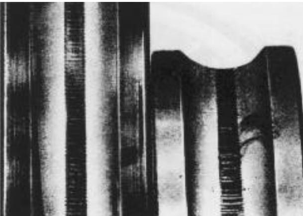
Fig. 3 Typical fluting damage to anti-friction bearings.
