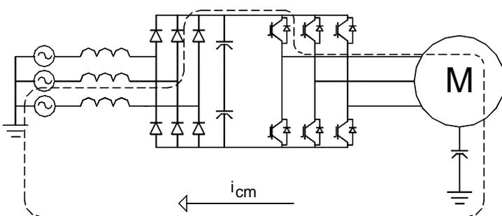
Fig. 8a Common-mode current flow in a conventional ASD and motor<sup>11</sup>
