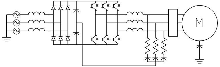
Fig. 8b Proposed output filter to reduce differential-mode and common-mode dv/dt at the terminals of the motor.<sup>11</sup>
