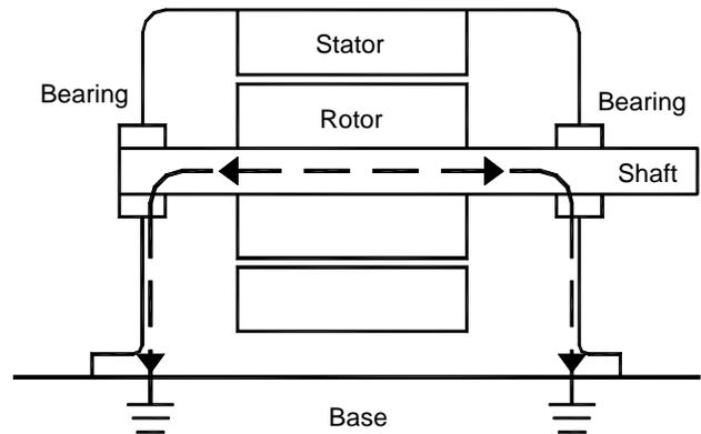
Fig. 2 Capacitively coupled current flow
