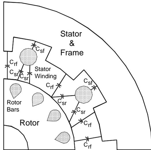
Fig. 4 Pictorial Diagram of Motor Capacitances<sup>5</sup>
