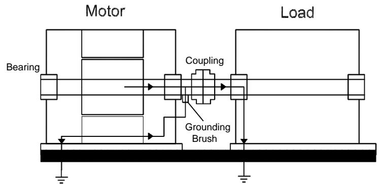
Fig. 7 Paths for common-mode currents to ground
